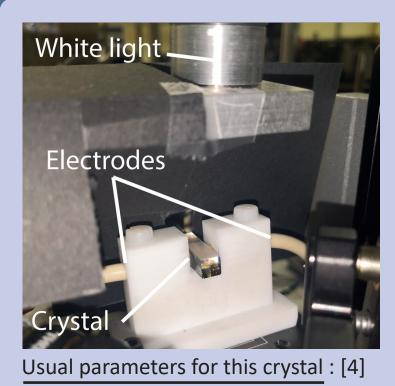
$n_0 = 2.36$  the refractive index of the crystal  $r_{33} = 250 \cdot 10^{-10} \, cm / V$  the electro-optic coefficient  $I_{sat} \sim 300 mW / cm^2$  the intensity of saturation  $E_0 \sim 1500V/cm$  the external electric field
