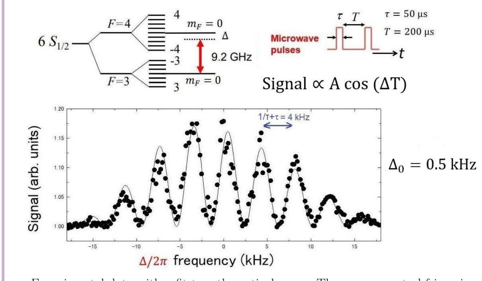
Experimental data with a fit to a theoretical curve. The narrow central fringe is centred on the nominal resonance.
