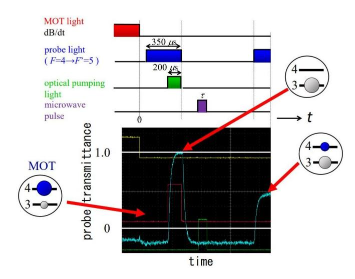
Example of a time sequence and probe transmission presented on the oscilloscope. This example is for just one microwave pulse (Rabi oscillations).
