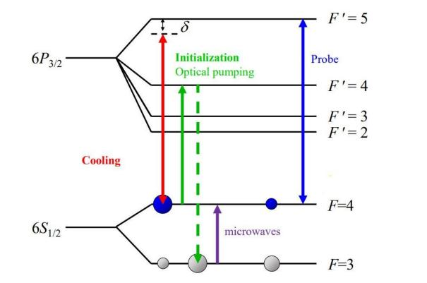
Energy diagram and transitions related to Rabi oscillations and Ramsey spectroscopy. The transitions shown in this diagram are presented in chronological order, from left to
