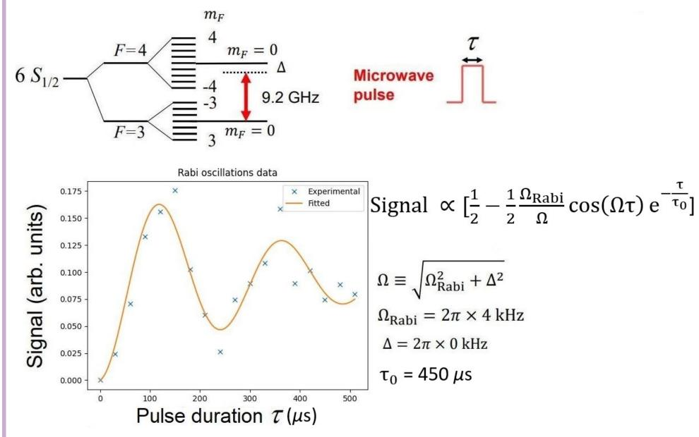
Experimental data and a fit in order to determine Rabi frequency and confirmation of the observation of the Rabi oscillations.
