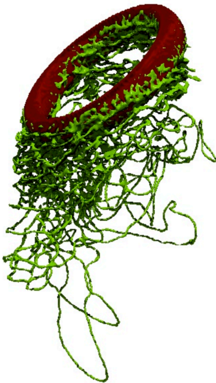
Vortex nucleation in the wake of an accelerated solid ring. Quantum vortices are the green filaments, and the object is displayed in red.
